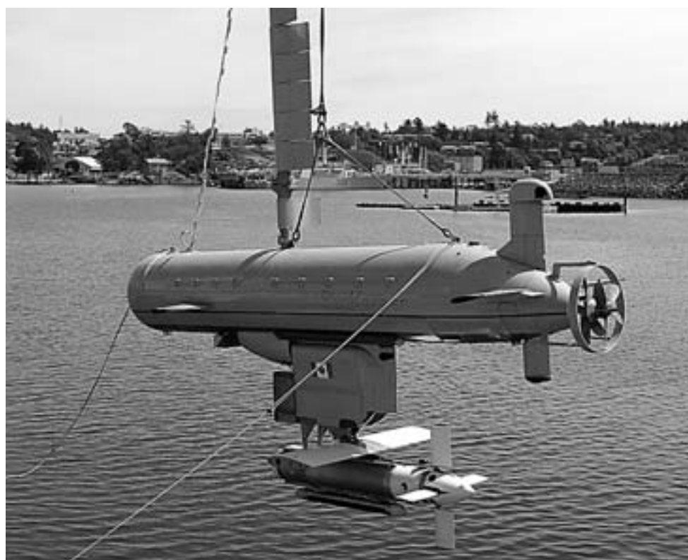
The semi-submersible, remote minehunting, vehicle called DORADO and its towfish before launching.
